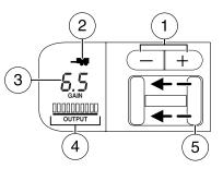
2. **Trailer connection indicator:** This lamp indicates trailer electrical connection status.
